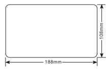
If the opening is too small, carefully cut or file as necessary until the radio easily slides into the opening. Do not force the radio into the opening. Check for sufficient space behind the dashboard for the radio chassis.
